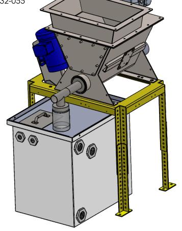
MAY FEED A HOLDING TANK OR AN EDUCTOR. 35 GALLON TANK SHOWN. OTHER SIZES ARE AVAILIBLE.
