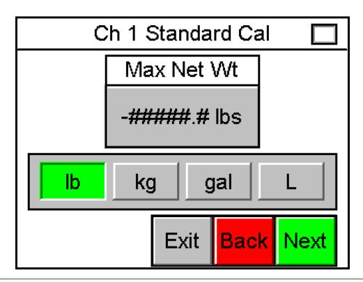
Figure 89: Standard Calibration: Max Net Weight
