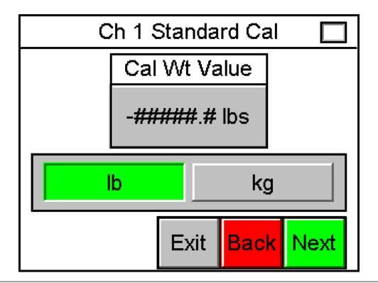
Figure 86: Standard Calibration: Calibration Weight Sample Success
