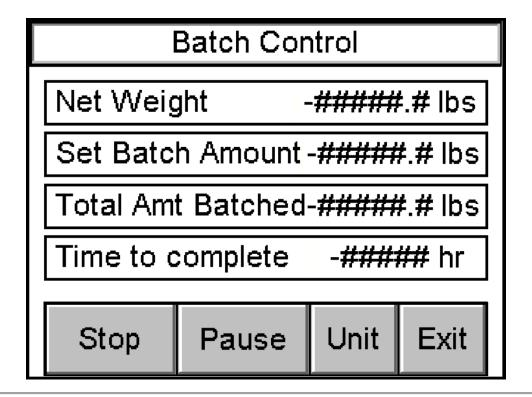
Figure 154: Batch Control Display
