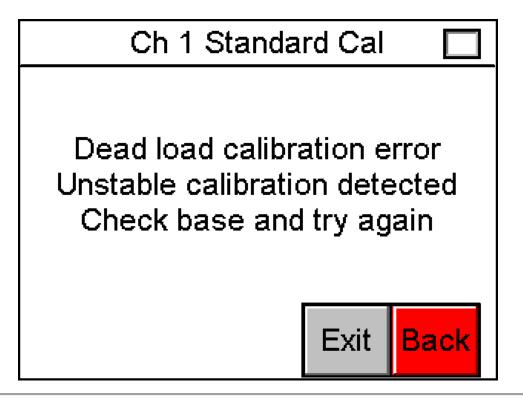
Figure 83: Standard Calibration: Dead Load Sample Error
