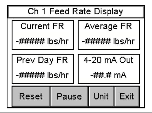
Figure 43: Channel 1 Feed Rate Display
