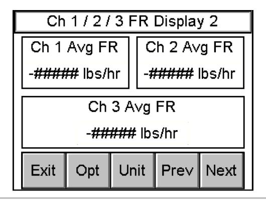
Figure 50: Channel 1 / 2 / 3 Feed Rate Display 2
