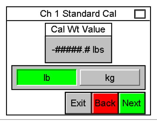
Figure 88: Standard Calibration: Calibration Weight Value
