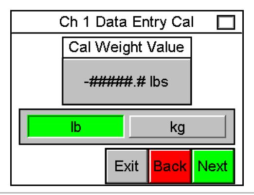
Figure 94: Data Entry Calibration: Calibration Weight Value
