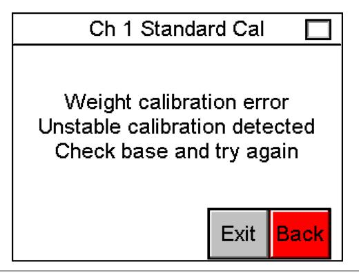
Figure 87: Standard Calibration: Calibration Weight Sample Error
